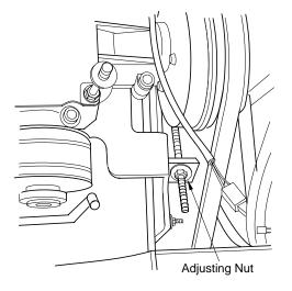
Figure 6-10 Blower Belt Adjustment
